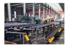
➤ Hot-Rolled seamless pipe production line for structural steel pipe, fluid conveying pipe, highand low-pressure boiler pipe, oil casing pipe and pipeline.
