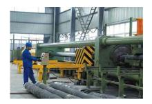
> SSAW & LSAW & ERW production line for large diameter welded pipe.
